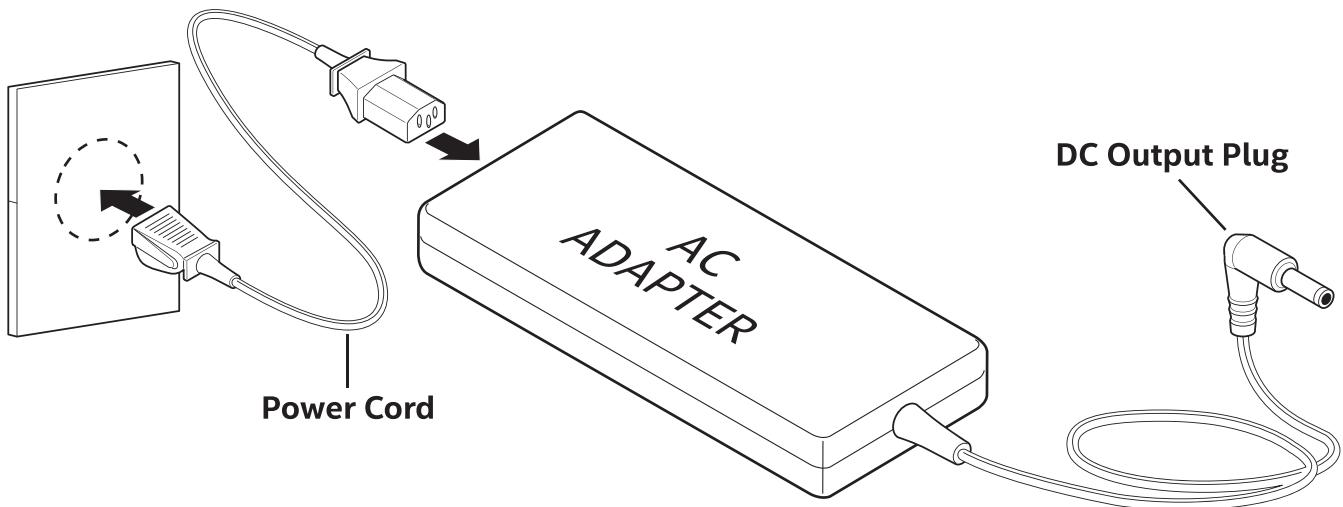
Connect the AC adapter's DC output plug to the DC IN jack on the back of the system.
