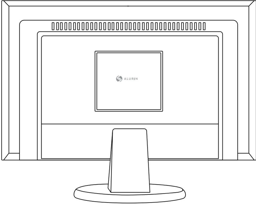
To assembly the mini Pc on the display, place the 4 screws on the mini Pc and then hang it from the back of the display.
